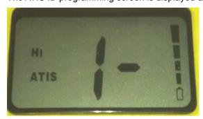
The left digit indicates the digit position of the ATIS ID; the right digit, which blinks continuously, indicates the value of that digit.
